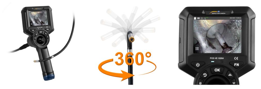
4-way industrial borescope with photo and video recording / 1280 x 720 pixels / 360° swivel / 6 mm (0.23") diameter / 1 meter (3 ft 2") cable length / LED lighting / Micro-SD card memory / Transport case / Battery life >3 hours / IP 67
