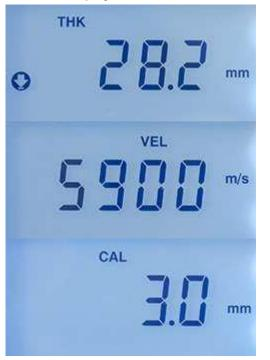
THK (thickness): material thickness measurement
