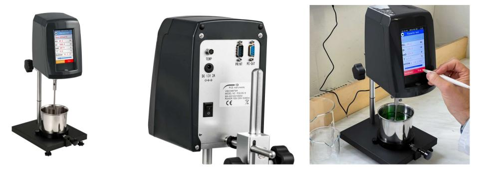
Viscometer / viscosity meter with PC interface / Optional ISO factory certificate / Touchscreen / Measuring units KU, cP, g / Measuring range 40.2 ... 141 KU / Height-adjustable stand mount / For measuring the viscosity of liquids / Overload protection / Optional software
