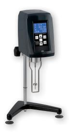
The viscometer has a measuring range of 1 ... 100,000 cP. With an accuracy of <±2% of the range, the viscometer is a precise measuring device to determine the viscosity of a sample liquid. The viscosity is determined by the viscometer on the basis of an applied mechanical resistance that acts in the opposite direction to the rotational movement of a spindle. The viscometer can be operated with an adjustable speed in the range between 6... 60 RPM.
