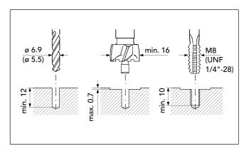
To drill the mounting hole, use drill bit 6.9 mm (M8) or 5.5 mm (UNF 1/4"-28). Torque and unscrew the transducer with a torque wrench and a 17 mm socket (SPM 81086).
