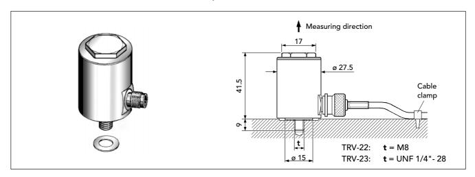
The transducers TRV-22 and TRV-23 are piezo-electric accelerometers of compression type, designed for vibration monitoring of industrial machinery. They can be used together with handheld instruments or in permanent installations. Max. cable length between transducer and measuring unit is 10 m (33 ft).
