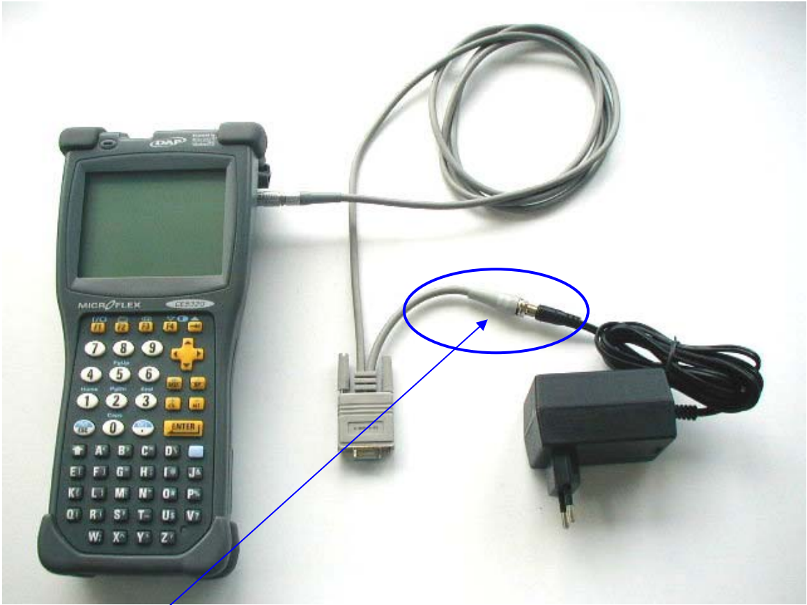
Figure b: how to connect the communication cable to the AD-adaptor cable
